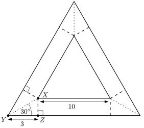
The symmetry of the involved equilateral triangles gives |YZ| = 3 and  $|\langle ZYX| = 30^{\circ}$ , and thus  $|XZ| = \sqrt{3}$ . Cutting the full body along the planes indicated in the picture above by dotted and dashed lines splits it into three cylinders of radius  $\frac{|XZ|}{2} = \frac{\sqrt{3}}{2}$  and height 10 and six pieces, which can be rearranged to form three cylinders of the same radius and height 3. The sought volume is thus
